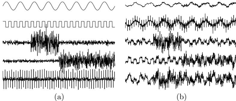
Figure 1: (a) Five artificial signals with simple frequency content (signals #1 and #2), simple on/off non-stationarity in time domain (signals #3 and #4) or quasi-periodicity (signal #5). (b) Five mixtures of the signals in (a).
